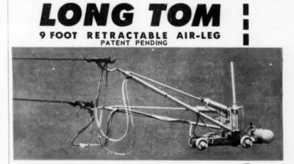
By adjusting the air pressure to the balancing cylinder the "Long Tom'' retractable air leg is held at any desired height, and movement up or down is accomplished simply by pushing down or lifting the leg (with one hand) to the new position.
